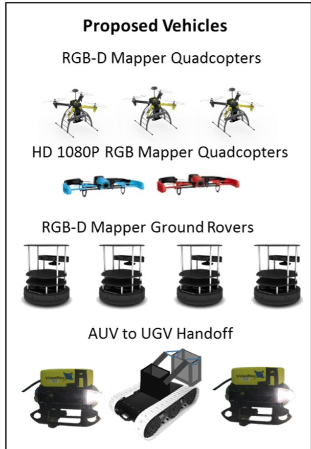
Fig. 2: Proposed Testbed Vehicles – Erle-Copters as the "RGB-D Mapper Quadcopters", Parrot Bebop UAVs as the "HD 1080P RGB Mapper Quadcopters" and Kobuki Turtlebot2s as the "RGB-D Mapper Ground Rovers"
