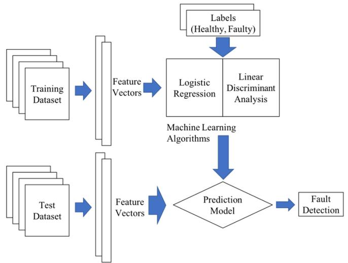
Figure 2: Block Diagram of Fault Detection Model
