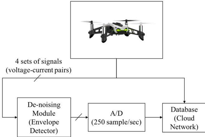
Figure 1: Block Diagram for Generating Dataset from actuator signals of the drone
