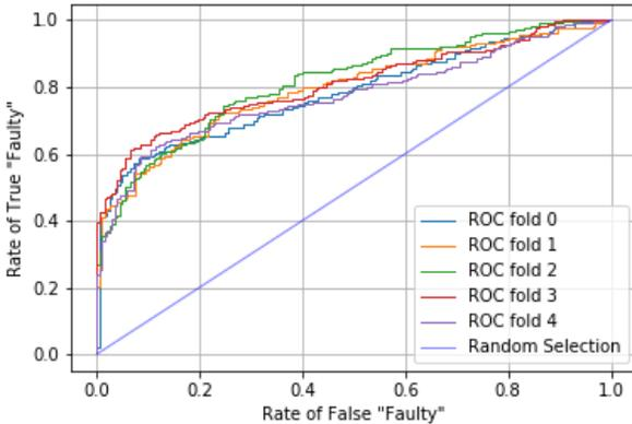
Figure 3: ROC plot of the data classification using LR
