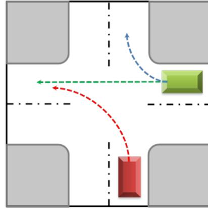
Fig. 1: Intersection driving scenario example. The green car has the right of way. The red car must know the green car’s intention to go straight or turn right in order to turn left safely.
