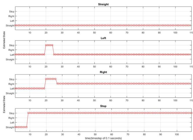
Fig. 6: Estimation of driver's intention at each timestep using four discrete HMMs for the different individual vehicle maneuvers including (a) Straight (b) Left (c) Right and (d) Stop.
