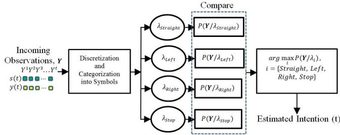
Fig. 4: Estimation of driver’s intention, that best represents the new observations sequences, using four discrete HMMs for the different driver intention including Straight, Left, Right and Stop.
