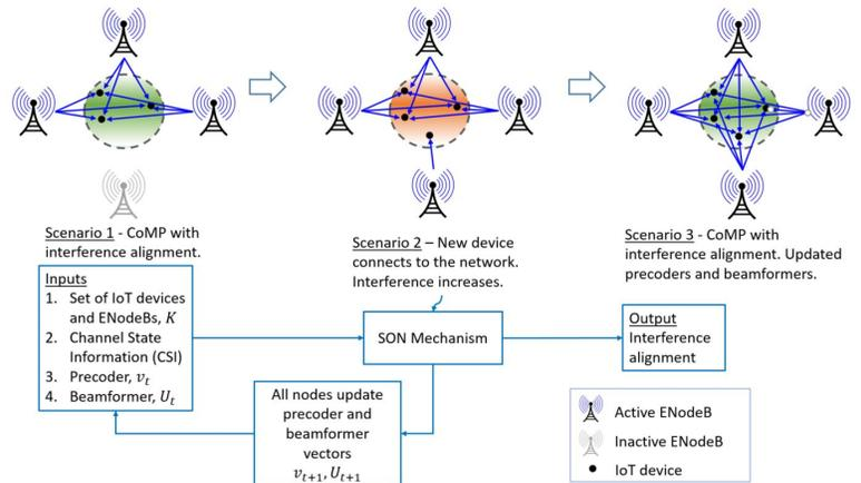
Fig. 4. SON protocol for interference alignment
