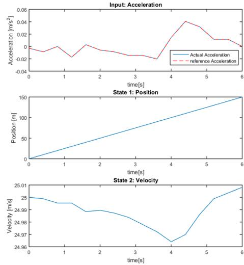
Fig. 6: Planned trajectory for subject vehicle in scenario 1
