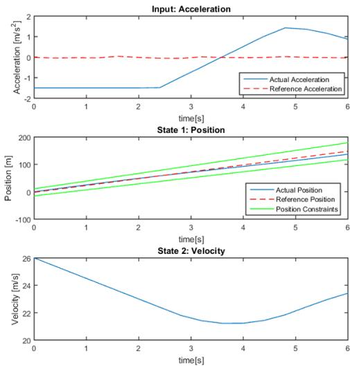
Fig. 7: Planned trajectory for subject vehicle in scenario 2 (in current lane)
