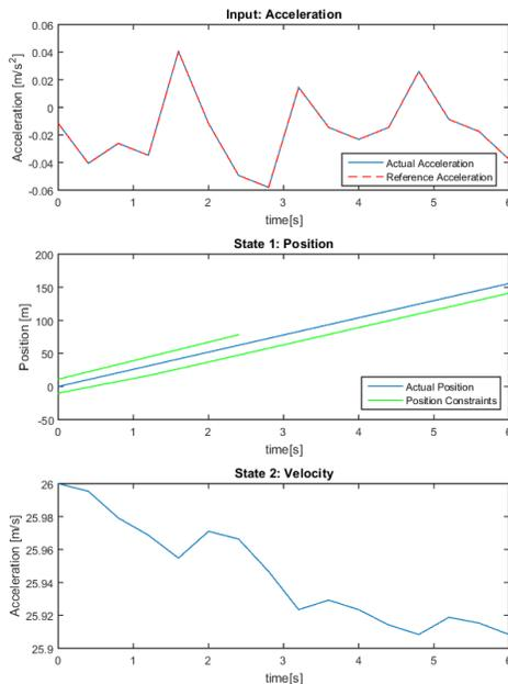
Fig. 8: Planned trajectory for subject vehicle in scenario 2 (in target lane)
