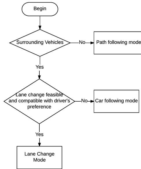
Fig. 1: Block diagram of the proposed algorithm
