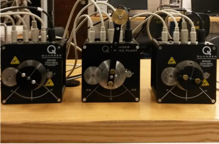
Figure 2: Setup of 3-agent system with disturbance; a flying mass is hanged to introduce disturbance
