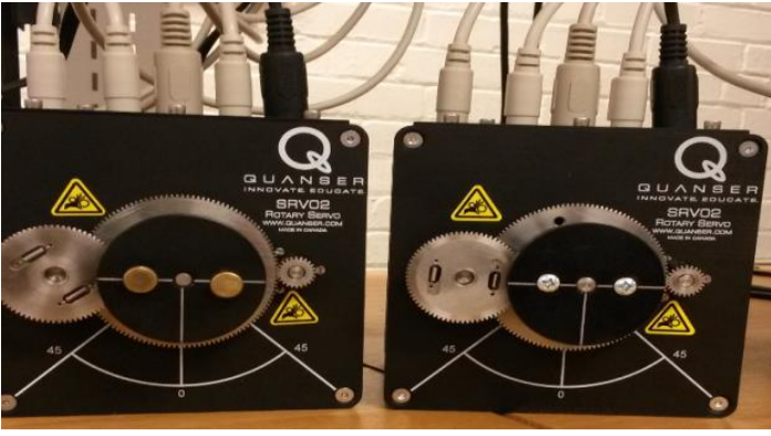
Figure 1: Two motor system; using angular motion sensors, state variables are collected
